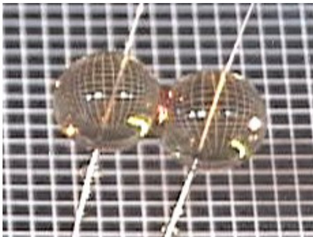
Two 1 ml liquid drops of honey in the process of coalescing to a single spherical drop.
