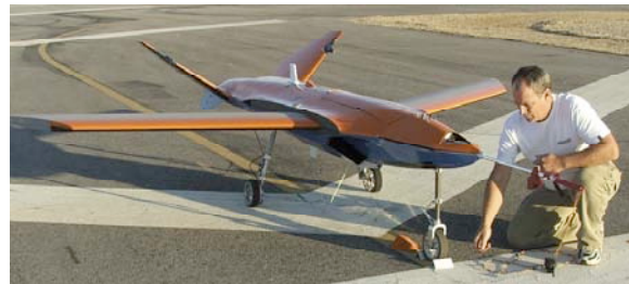
Figure 7 Morphing RPV Developed by NextGen Aeronautics in the DARPA MAS III Program
