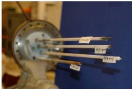
Anode Electrode Lost in Melt
