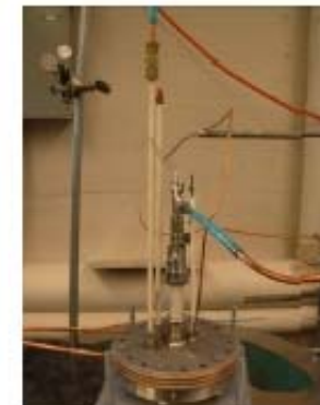
Furnace cap with O 2 collection device
