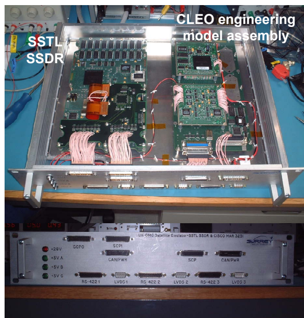
Figure 3.—CLEO ground-based testbed. (a) Top view, before adding fans and heatsinks. (b) Front view of ports.
