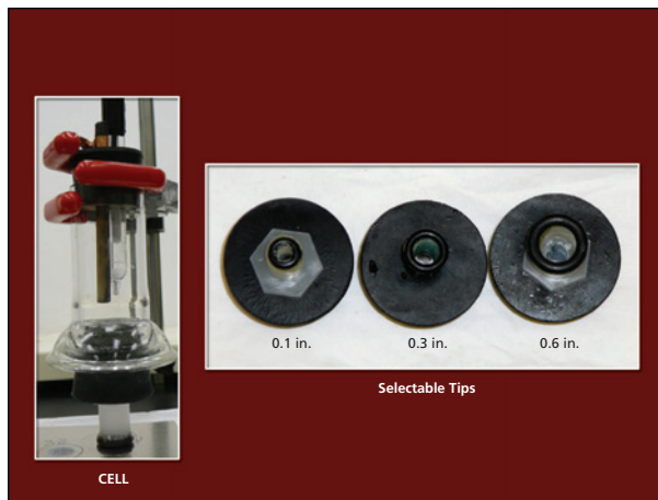
This Corrosion-Testing Electrochemical Cell is equipped with one of three selectable tips. Each tip features a different corrosion-pit diameter.
