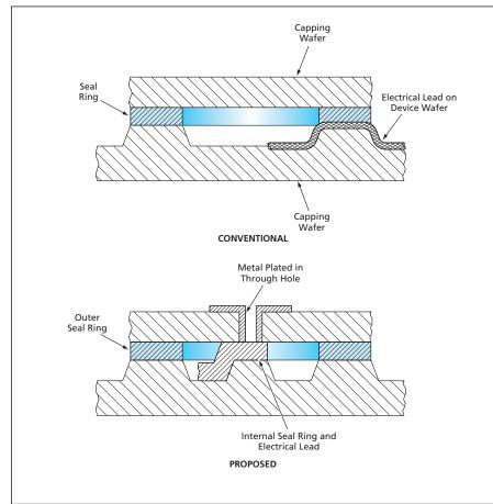
These **Cross Sections of Pertinent Parts** of one of many identical devices fabricated on a wafer are greatly simplified in order to illustrate salient differences between the proposed method and the conventional method.
