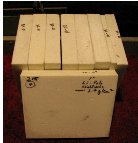
Figure 6: Sample coupons of lithium doped polyethylene (92.5% polyethylene, 7.5% lithium). The samples had dimensions of 15.24 cm x 15.24 cm (6" x 6") and the blocks were of various thicknesses. There are a total of ten coupons.
