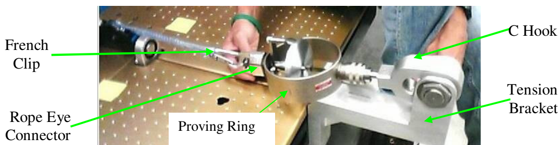
Figure 16. ARED Calibration Tool Installed for Tension Load Cells
