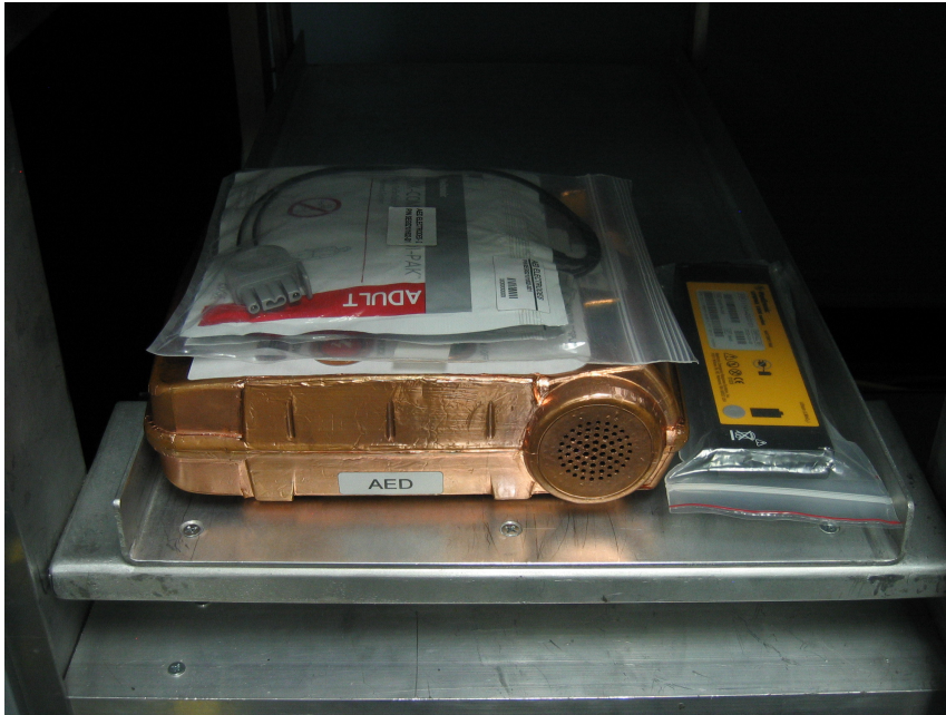
Figure 3. AED Storage Configuration
