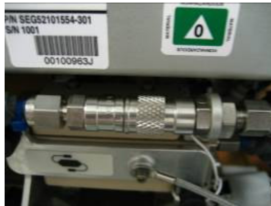
Figures 23-24. Incorrect and Correct QD Connections, Respectively
