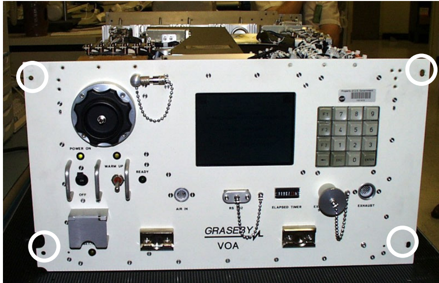
Figure 3. VOA Front Panel (CHeCS Rack attach points at corners)
