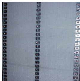
Figure 3. Belt Underside with Weld Nuts
