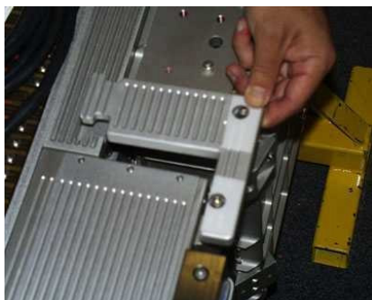
Figure 5. Forward Closeout Panel
