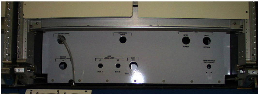
Figure 8. CHeCS Rack: Utility Interface Panel
