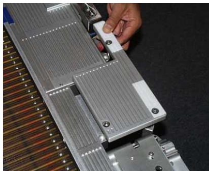
Figure 6. Aft Closeout Panel
