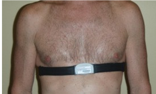
Figure 5. Correct Transmitter Placement
