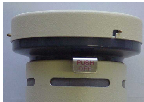
Figures 7-8. Microbial Air Sampler PUSH ON and PUSH OFF Sliding Valve (Rocker switch)
