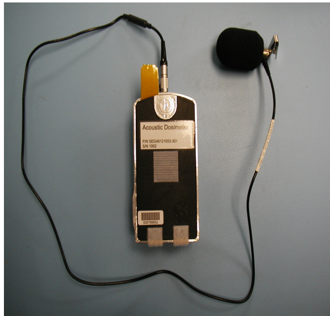
Figure 11. - Protective Cover on Acoustic Dosimeter
