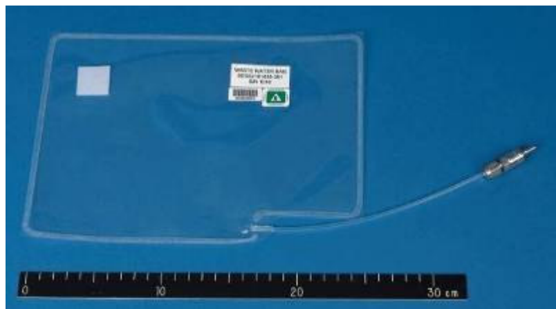
Figure 5. TOCA Waste Water Bag
