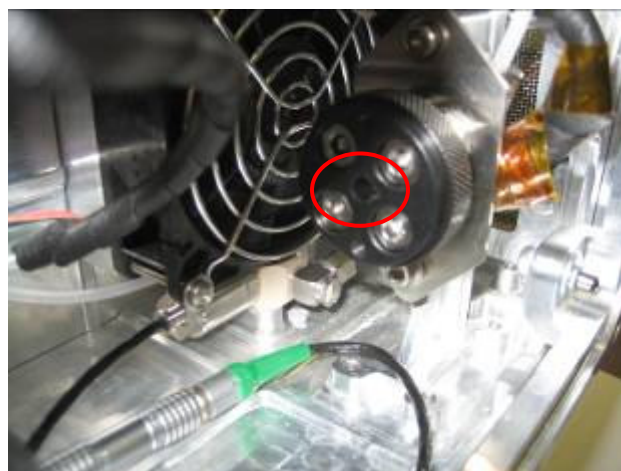
Figures 19-20. Gas Liquid Separator, Location to be Installed
