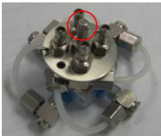
Figures 19-20. Gas Liquid Separator, Location to be Installed
