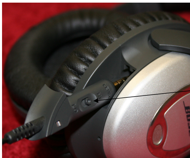
Figure 3 - Hi/Lo Switch on Audio Cable
