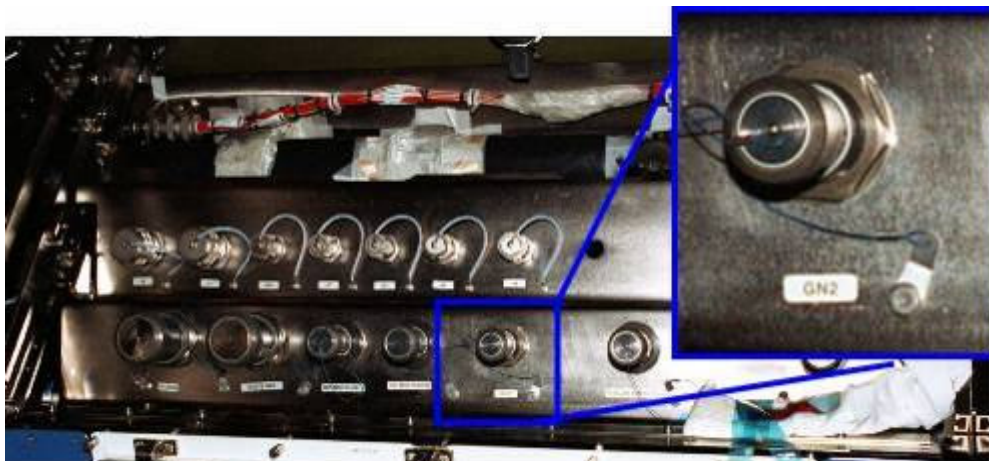
Figure 18. GN 2 QD Connection at Z Panel
