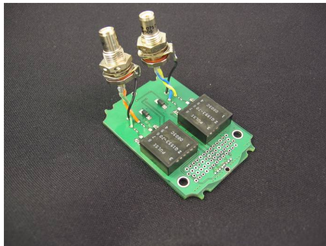
Figure 14: External Connectors are mechanically decoupled via “Flying Lead” connections for all PIM I/O as well as for the console port connector.
