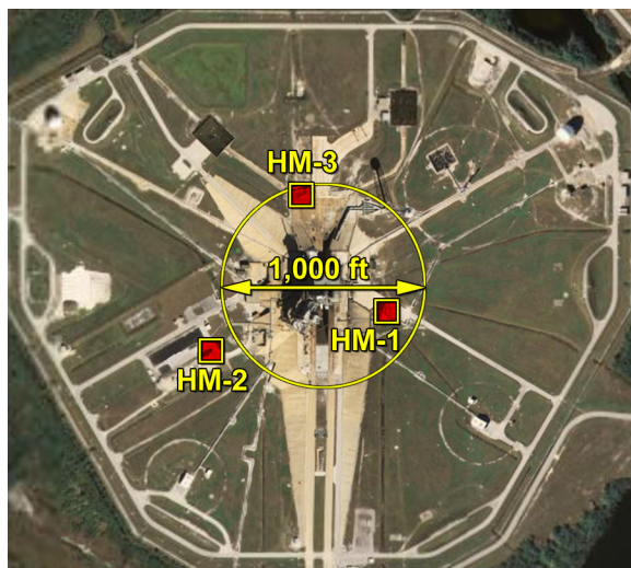
Location of hail monitor stations, HM-1, HM-2, and HM-3, at Launch Pad 39A.
