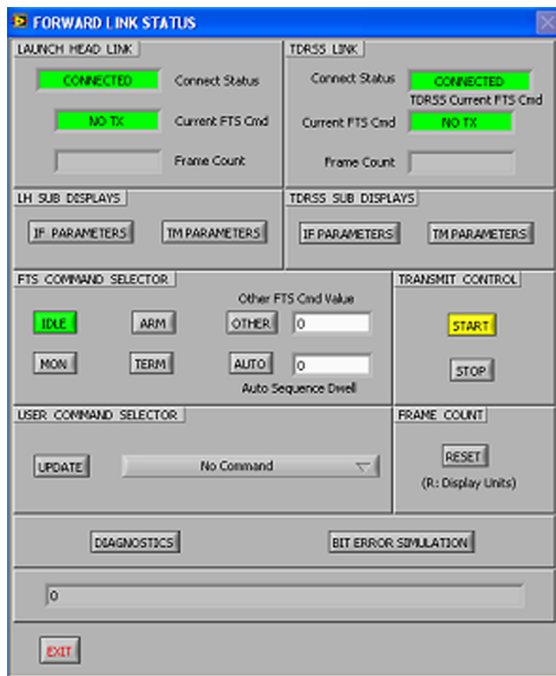
Telemetry workstation forward-link status display.
