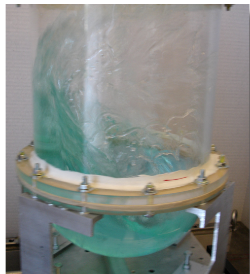
Slosh induced in test tank.
