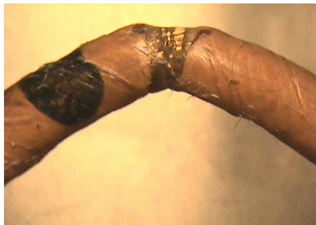
Figure 1. Small, compact repairs on 12-gauge insulated wires exhibit excellent flexibility.
