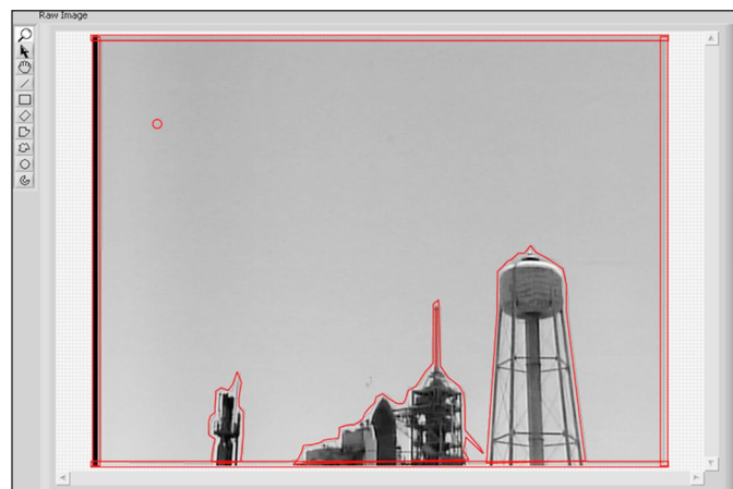
Manually drawing exclusive regions of interest helps mitigate false detections from background noise.
