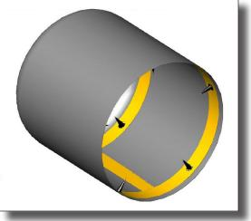
Tank instrumented with low-gravity probes.
