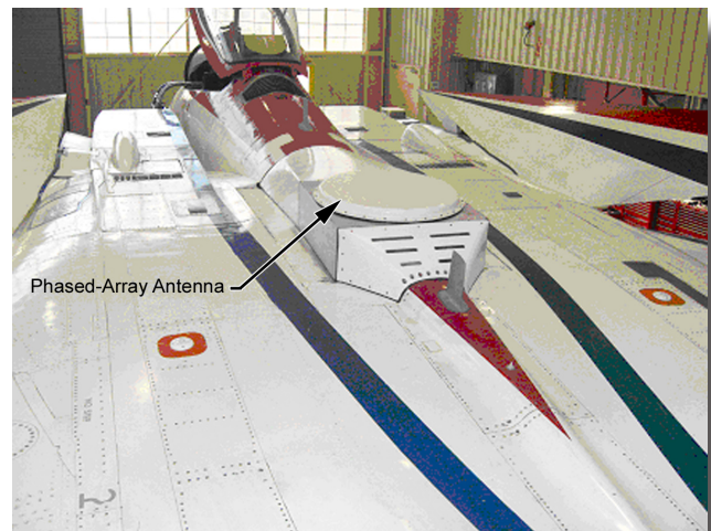
Figure 3. Phased-array antenna on the F15.
