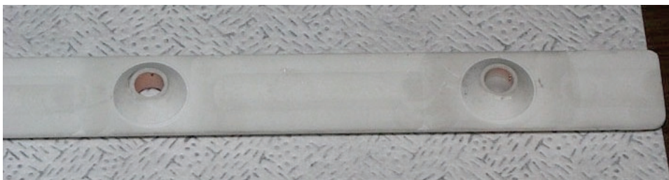
Fig. 6. Standard source lid with conical nozzles used for all the metal evaporation sources in the system.
