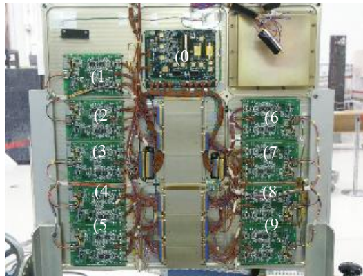
Figure 4: Photograph of the DAC boards (1-9) and main microprocessor board (0) that perform the FTSCE electrical measurements. The metal box in the upper right of the photograph is the power control unit (PCU). The metal boxes in the center route wires from the solar cells mounted on the opposite side and serve to maintain a Faraday cage around the measurement electronics.
