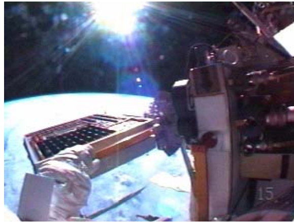
Figure 8: A still shot from Astronaut Soichi Noguchi's helmet camera showing him deploying MISSE5 on the top of the ISS P6 truss
