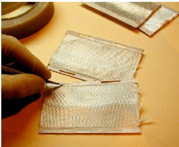
Figure 5. UV Rigidizable Hinge Manufacturing
