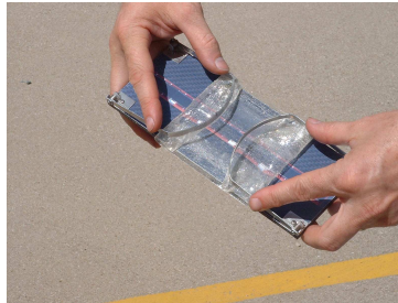
To Prove the Concept, ENTECH Built This Model Last Year Using a SCARLET Lens "Coated" with a 75-Micron-Thick Glass Arch, Broken into Small Pieces to Simulate the Parquet
