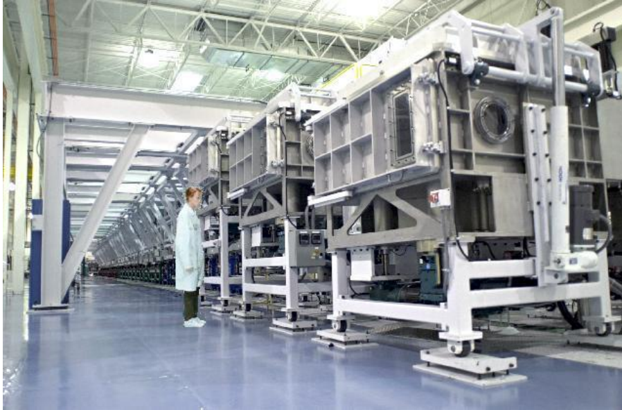
Figure 2. The roll-to-roll a-Si deposition machine for terrestrial products with 25 MW/year capacity.
