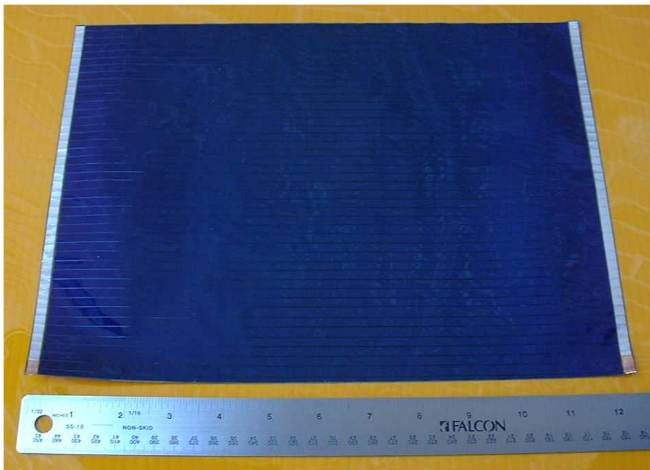
Figure 9. A production size cell on 1 mil polymer with total area 23.88 cm x 32.08 cm.
