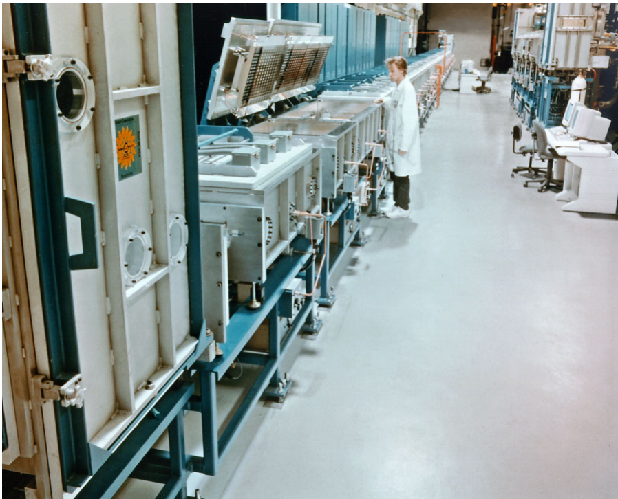
Figure 3. The roll-to-roll a-Si deposition machine previously used for terrestrial products with 5 MW/year capacity, now dedicated to research and production of space cells.
