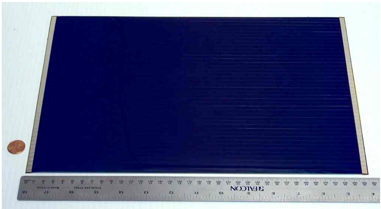
Figure 6. An L-strip with 806.5 cm 2 aperture area on ~ 1 mil stainless steel.
