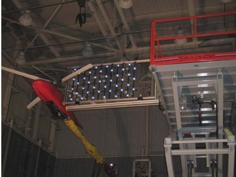
Figure 18. Three-dimensional calibration target positioned in measurement plane.
