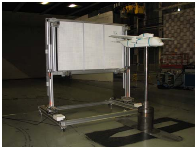
Figure 4. Target used to calibrate the LFPIV system.
