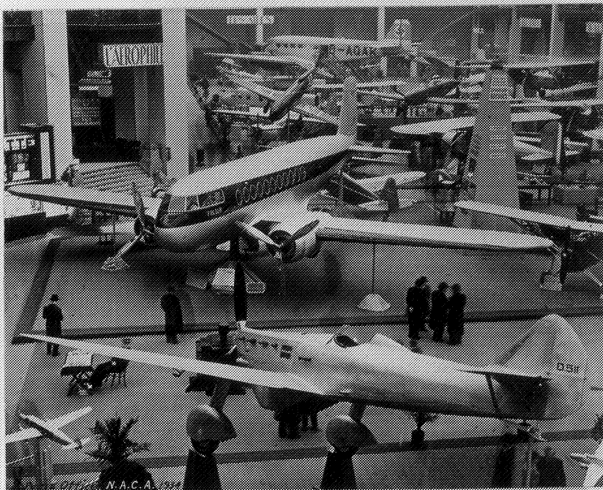
Figure 6.— Dewoitine D 511 pursuit monoplane. 850 hp. Hispano-Suiza engine. 1 20 mm cannon. 2 machine guns. (in foreground) Breguet 46 transport monoplane. (in background)
