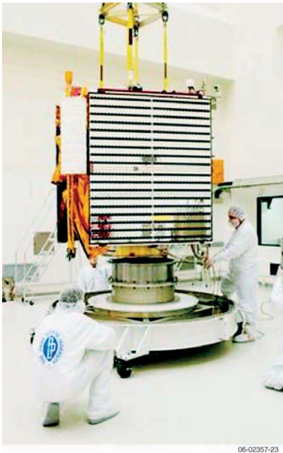
Figure 4-23. MESSENGER solar panel showing the use of OSR to maintain array operating temperature within acceptable limits.
