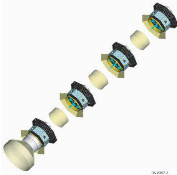
Figure 4-3. The four IHS spacecraft and three interspacecraft support structures in the stacked configuration.
