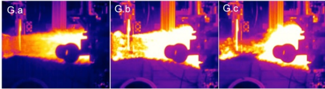
Figure 12. Cases G.a, G.b, G.c, M_h=6 and H_2 or mixed H_2-C_2H_4 coflow, showing detachment as H rate is decreased.
