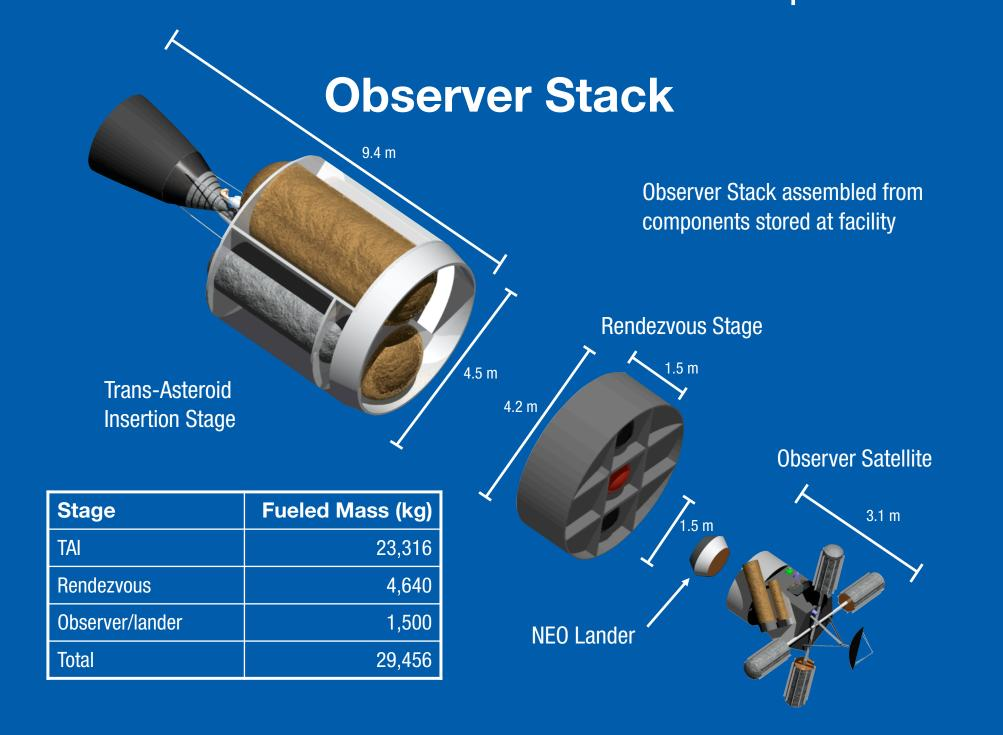
The observer stack can be launched on a number of existing and proposed launch vehicles. Some non-U.S. vehicles may have the needed performance as well.
