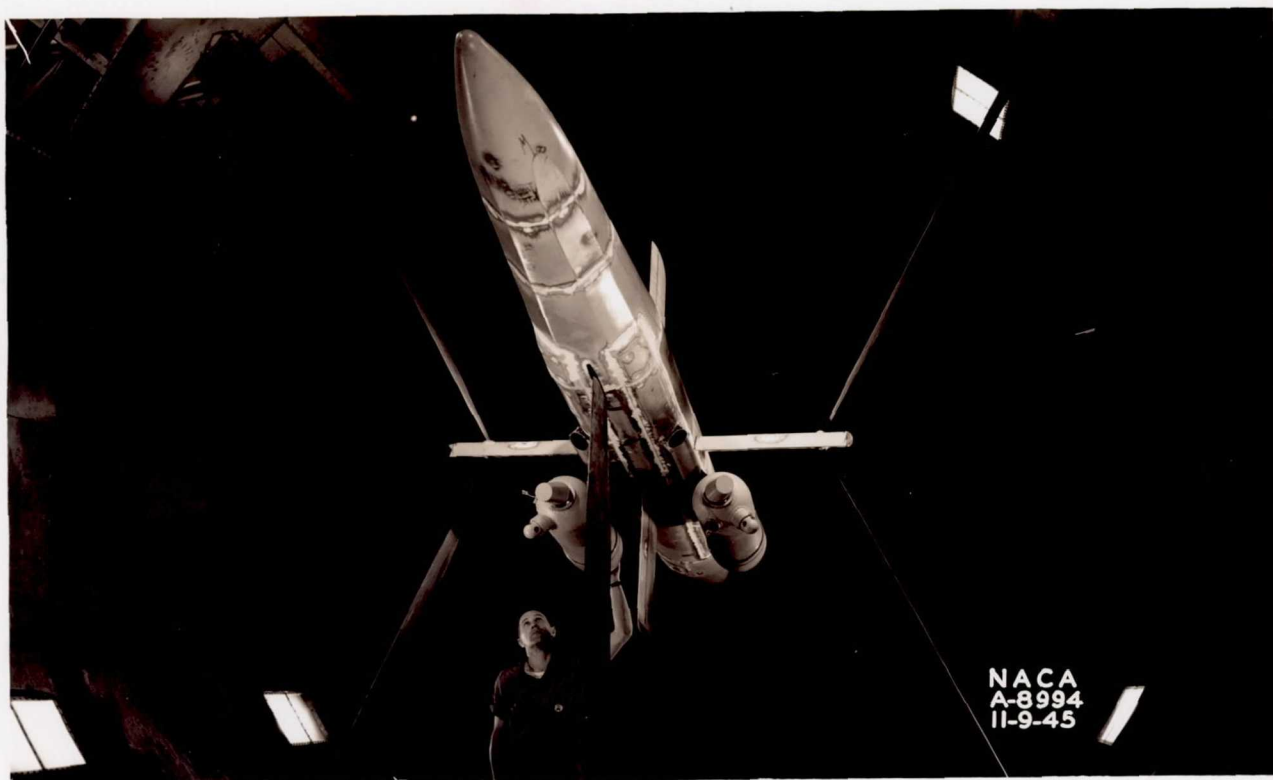
(d) Rear view of the model, less tail surfaces, with the jatos attached and with the standard lower rear strut.
