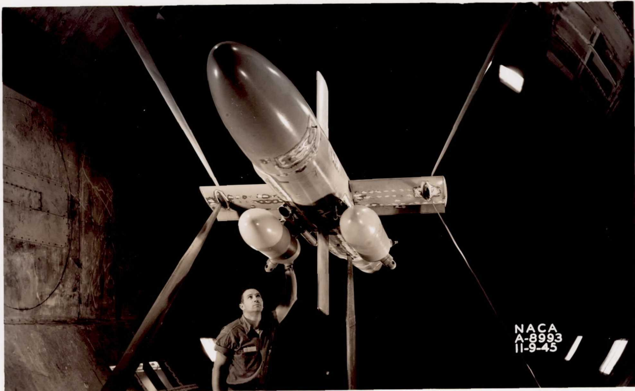
(c) Front view of the model, less tail surfaces, with the jatos attached and with the standard lower rear strut.
