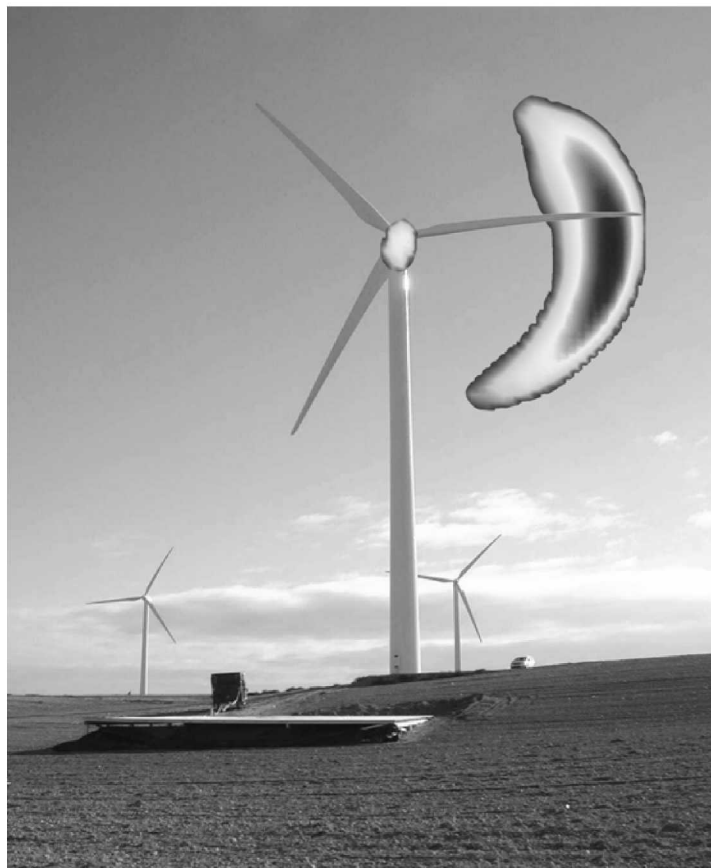
Figure 7-44. Noise sources measured on a Gamesa G58 850 kW wind turbine by means of a microphone array on the platform in the foreground. The downward-moving blades emit the majority of the noise, as indicated by the sound power contours whose range is 12 dB. [Oerlemnes 2005]
