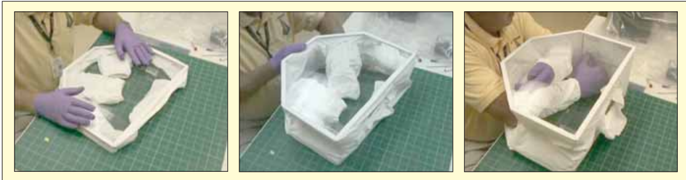
Only Simple Motions are needed to prepare the glove box for use.
