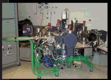
Uses secondary ions from sample surfaces to identify elements and their isotopes Sensitive to all elements and crystal impurities at ppm levels. Can map all elements, including hydrogen. Incorporates elemental distribution, depth profiling, and quantitative analysis. Requires flat polished samples and very high vacuum.
