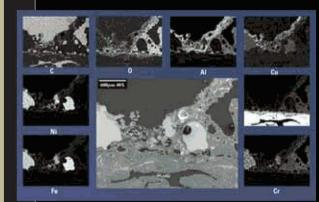
Identify elemental distributions in slag using SEM with x-ray mapping.
