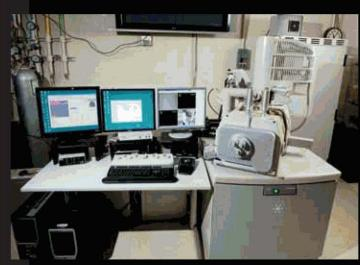
Provides very high resolution and depth of field. Can examine metallic, nonmetallic, and wet samples, up to 12 inches wide. Uses EBSD to evaluate grain orientations. Resolution 2nm@30KV, magnification 7X to 1MX, maximum pressure 20 Torr. Particle analysis systems, SDD energy dispersive spectrometry (EDS).
