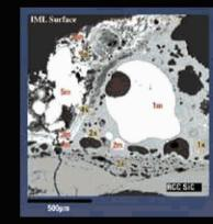
Identify precise quantitative chemical composition of slag feature, using electron microprobe
