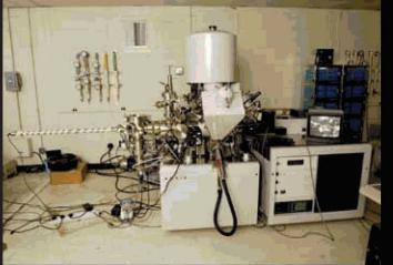
Uses white/monochromatic X-rays for surface chemical analysis, including depth profiling. Can identify elements and their chemical states. mapping, imaging, and identifying compounds, films, and
