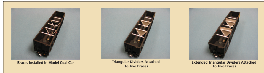
Figure 1. Triangular Dividers can be attached to triangular braces in a typical coal car to reduce aerodynamic drag when the car is empty.
