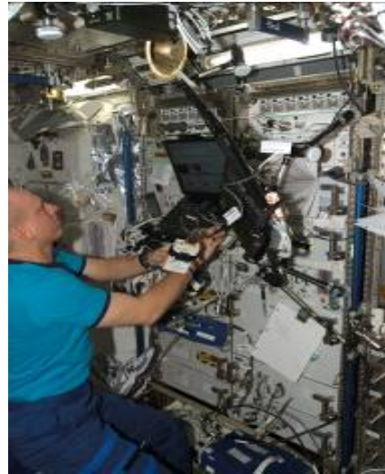
ISS015E14753 - Expedition 15 Flight Engineer Clay Anderson is seen here working with an Actiwatch reader and computer during hardware setup for the CCISS experiment in the U.S. Laboratory Destiny . The continuous blood pressure device (CBPD) is also visible in the background.
