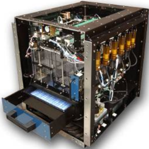
The avian hatching habitat with the exterior panels removed.
