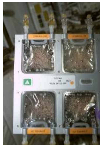
ISS004E5210 — Image of the Quad Tissue Culture Module Assembly (QTCMA)-5 on ISS Expedition 4 after activation of the cells. A syringe was used to inject cells into the pink nutrient growth media. When the samples completed their growth cycle, the crew transferred the cells from the incubator to the biotechnology refrigerator, where they were stored until they were examined at a ground-based laboratory.
