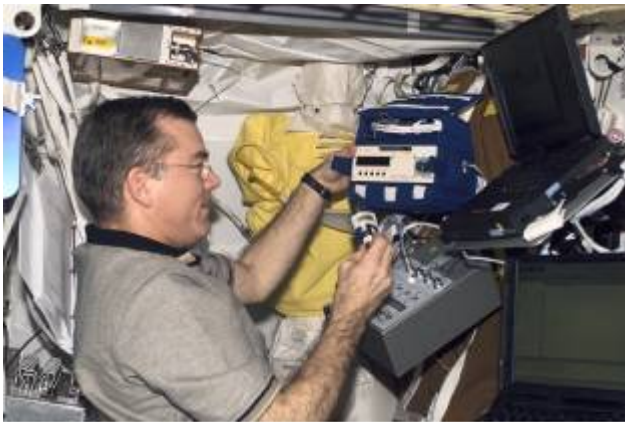
ISS002E7814 — James S. Voss, Expedition 2 flight engineer, sets up the HRF DOSMAP power distribution unit in the U.S. Destiny laboratory.
