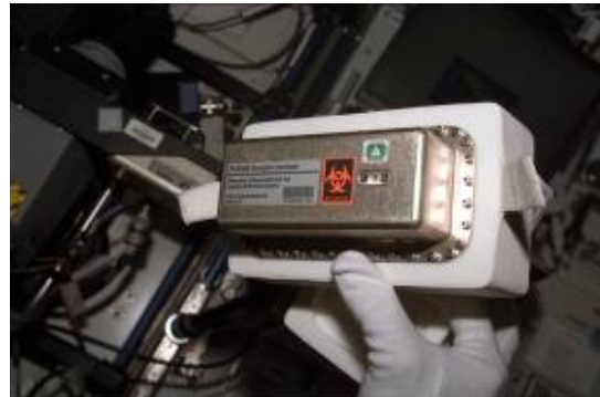
ISS014E05120 — Astronaut Michael E. Lopez-Alegria, Expedition 14 commander and ISS science officer, prepares to work with a POEMS sample container in the Destiny laboratory module.
