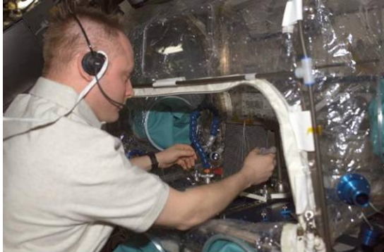
ISS009E14560 — Mike Fincke, Expedition 9 science officer, is shown deploying one of the drops of liquid onto Nomex thread during FMVM testing.
