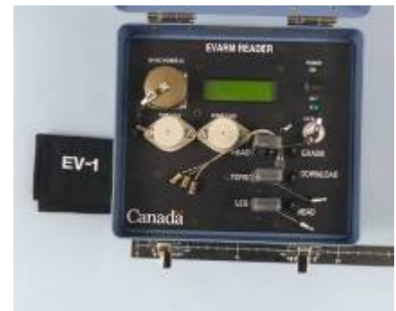
EVARM hardware. The device shown records and processes data sent by radiation detectors in the spacesuits of spacewalkers during EVAs.
