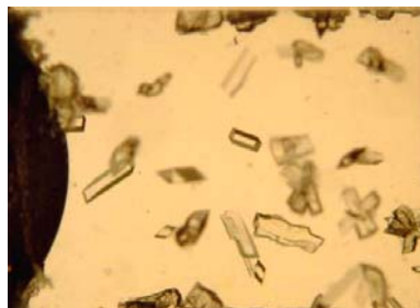
Camelid crystals, complexed with lysozyme, grown in the APCF during ISS Expedition 3.
