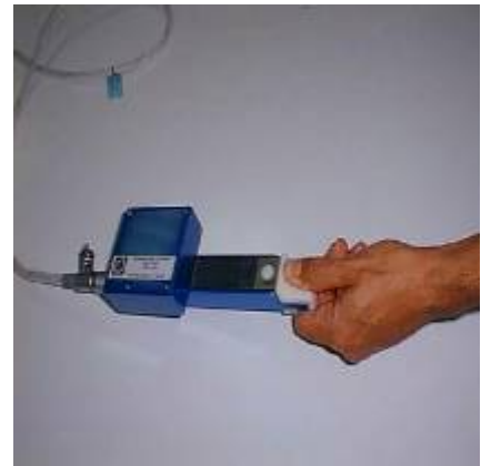
Hand grip dynamometer that was used for the muscle fatigue experiment that was part of the HPA investigation on board station.
