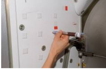
ISS014E18794 — Expedition 14 Flight Engineer Suni Williams uses the swabbing unit to collect samples that will be placed into the cartridges to be analyzed by the LOCAD reader.
