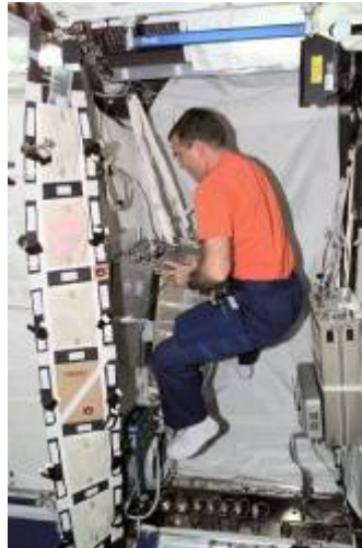
ISS002E5714 — Astronaut James S. Voss, Expedition 2 flight engineer, sets up the BBND inside the U.S. Destiny laboratory. He holds the control unit (nearest the wall) and the detector unit (DU) (in his hands).
