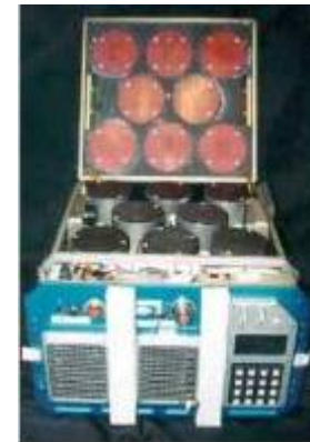
CGBA ICM with eight containers. The ICM provides both the computer and the thermal control for the samples.
