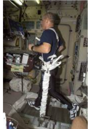
ISS006E11018 — Expedition 6 commander Kenneth Bowersox, wearing a body harness, runs on the TVIS as part of the Foot experiment in the Zvezda service module.
