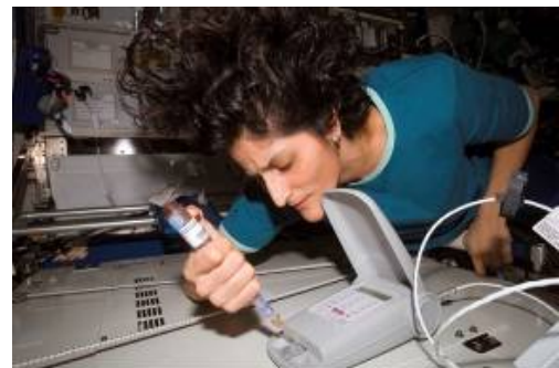
ISS014E18822 — Astronaut Suni Williams, Expedition 14 flight engineer, works with the LOCAD-PTS. Williams is placing the sample mixed with water from the swabbing unit into the LOCAD-PTS cartridge.
