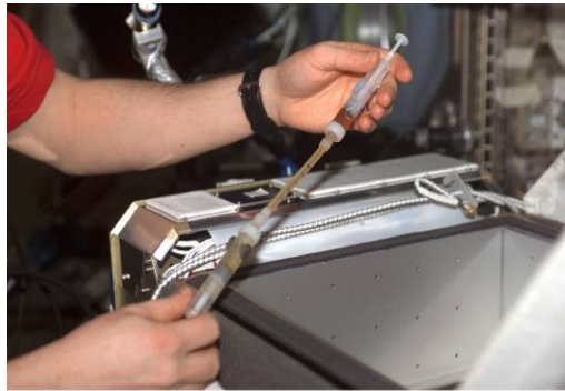
Edward M. (Mike) Fincke, Expedition 9 science officer and flight engineer, uses syringes to inject honey into water to test the mixing ability of the two liquids for the MFMG experiment.
