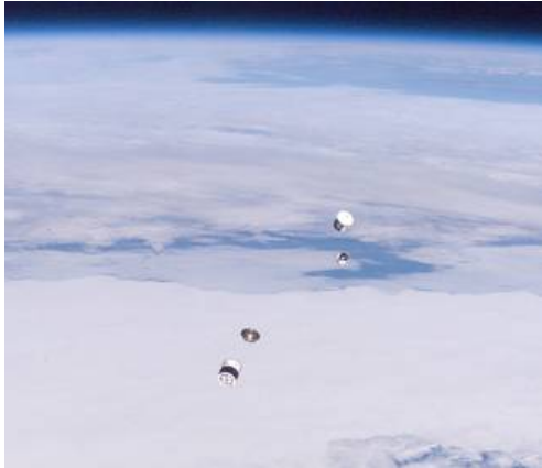
S116E07836 — Shown is one of the ANDE satellites floating free from the internal cargo unit (ICU) after deployment. The second satellite did not leave its half of the ICU until 4 hours later.
