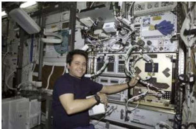
ISS004E11048 — The CGBA isothermal containment module (ICM) v.3, installed in ExPRESS rack just above astronaut Dan Bursch's extended left arm; photograph taken during Expedition 4.
