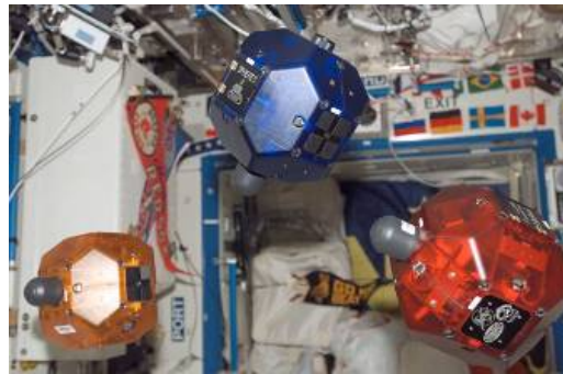
ISS014E17874 — Three satellites fly in formation as part of the SPHERES investigation. This image was taken during Expedition 14 in the Destiny laboratory module.
