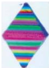
A thaumatin crystal, grown in microgravity during Expedition 3, displays interference patterns in polarized light.
