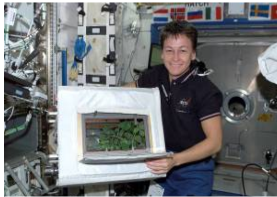
ISS005E07209 — Astronaut Peggy A. Whitson, Expedition 5 NASA ISS science officer, displays a first crop of soybeans growing inside the AdvAsc. Photos of the growing plant have been a useful tool for the ground-based science team, which uses them to determine optimal time for cross-pollination and harvesting.
