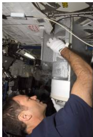
ISS014E05124 — Expedition 14 commander and NASA science officer, Astronaut Michael E. Lopez-Alegria, is shown inserting a sample container for the POEMS payload in the MELFI in the Destiny laboratory of the ISS. MELFI is a low-temperature freezer facility with nominal operating temperatures of -80^{\circ}\text{C} ( -112^{\circ}\text{F} ), -26^{\circ}\text{C} ( -15^{\circ}\text{F} ), and 4^{\circ}\text{C} ( 39^{\circ}\text{F} ) that will preserve experiment materials over long periods.
