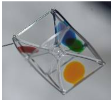
ISS006E18432 — View of surface tension demonstration during Saturday Morning Science, using water that is being held in place by a metal loop. Food coloring has been added to the water for demonstration purposes only.
