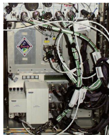
ISS003E8171 — Close-up image of DCPCG hardware, the V-locker, and the C-locker in ExPRESS Rack 1 on ISS Expedition 3.
