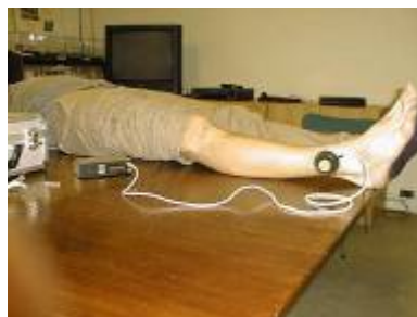
A Xenon detector unit is attached to each crewmember's leg, slightly above the ankle, as shown here.
