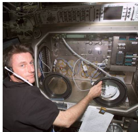
ISS008E06301 — C. Michael Foale, Expedition 8 mission commander and ISS science officer, installs equipment in the MSG for the PFMI experiment.
