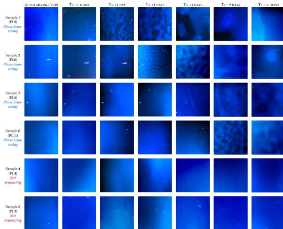
Images of BCAT-3-4-CP: Six samples of colloid/polymer mixtures separating at different times.
