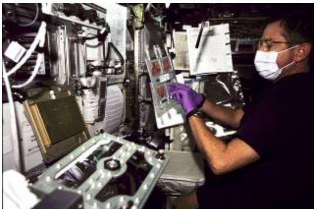
ISS003328030 — Frank L. Culbertson, Jr., Expedition 3 mission commander, works at the biotechnology specimen temperature controller (BSTC) for the CBOSS in the U.S. Destiny laboratory on ISS.
