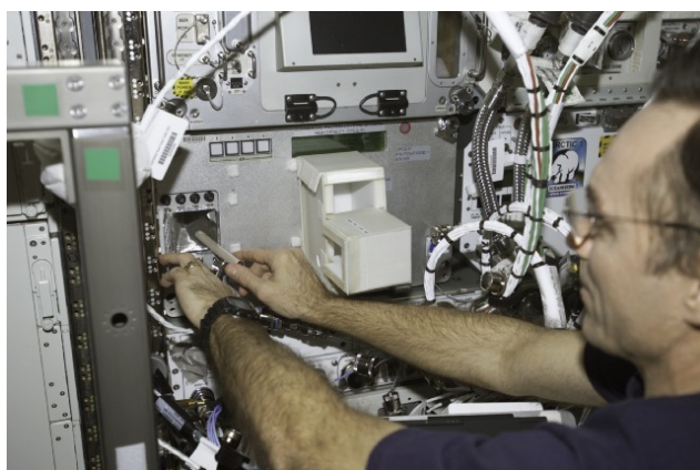
ISS004E10827 — Astronaut Carl E. Walz, Expedition 4 flight engineer, works in the U.S. Destiny laboratory installing the CRIM-M. CRIM-M provides the temperature control that is critical to the success of CPCG-H experiments.
