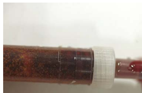
ISS011E07771 — Close up view of the MFMG syringe containing honey that is injected with tinted water during Expedition 11.
