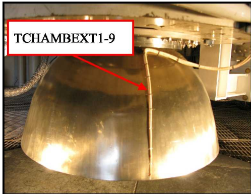
Figure 11: Dual-Bell Nozzle Thermocouples
