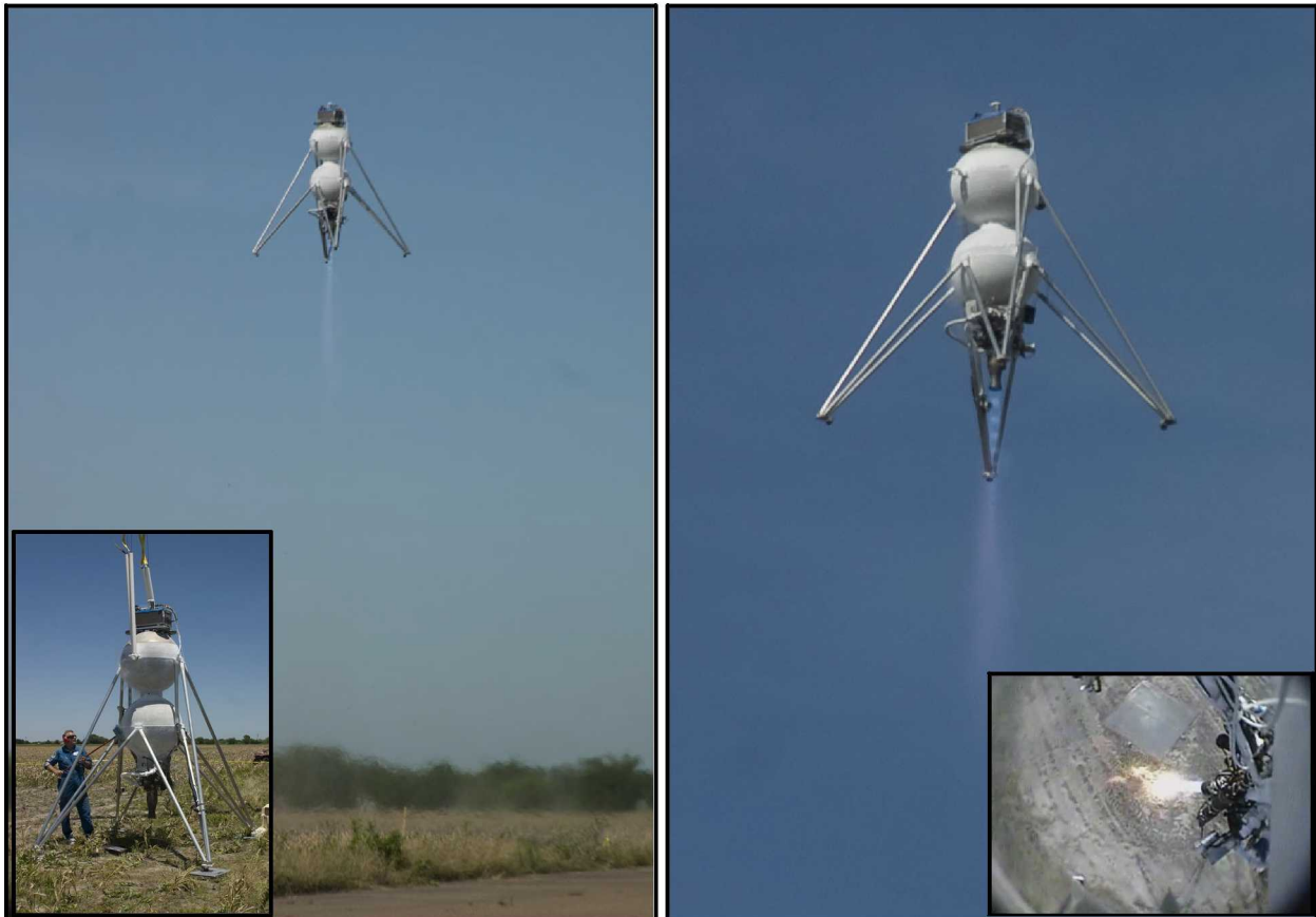
• Figure 1: Armadillo Aerospace VTOL Modular Vehicle in Typical Un-Tethered Flight Testing
