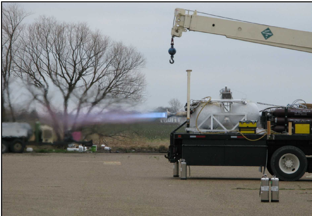
Figure 5: Armadillo LO 2 / LCH 4 engine test on horizontal test sled at full throttle
