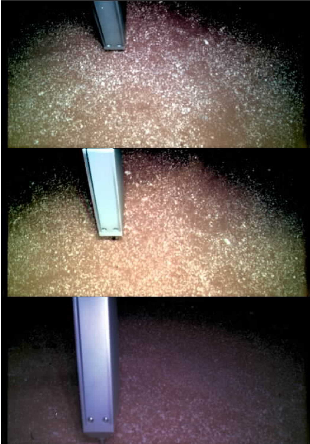
Figure -16. The RAC view of the TECP at insertion angles of 30°, 47° and 77° (top to bottom).
