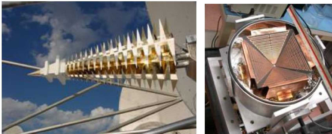
Figure 4-2. Left: ATA feed installed on an ATA dish. Right: Prototype Eleven feed in a cryogenic dewar.
