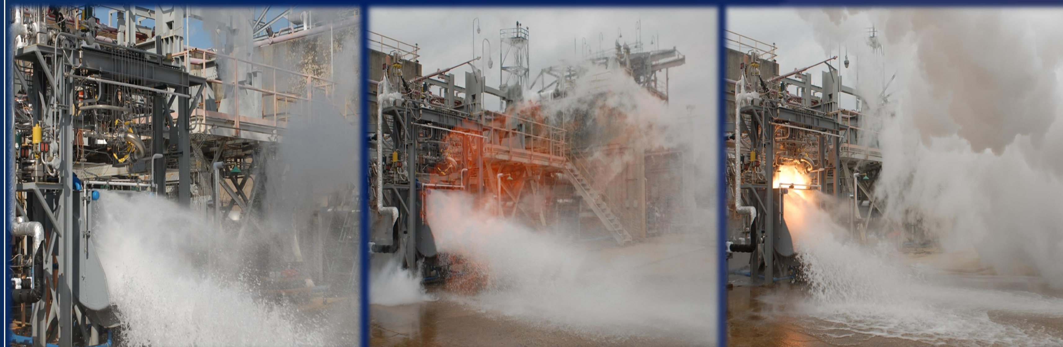
J-2X Workhorse Gas Generator Firing
