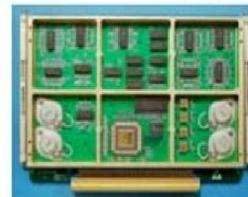
Built Up Data Acquisition System (DAS) Module
