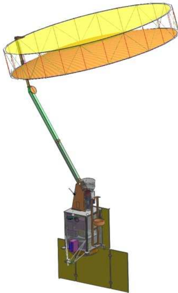
Fig. 1 The SMAP observatory is a dedicated space-craft with a rotating 6-m light-weight deployable mesh reflector. The radar and radiometer share a common feed.
