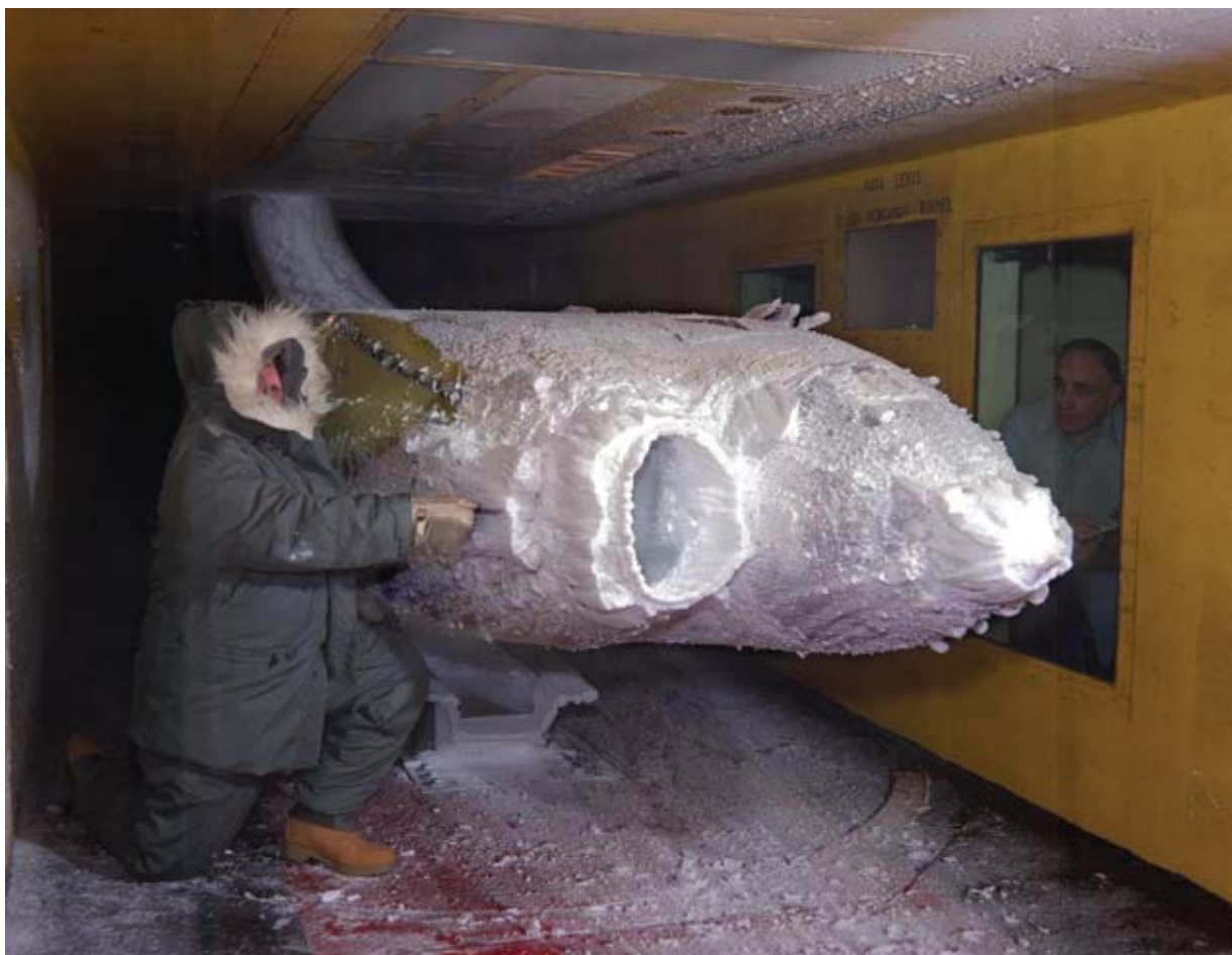
Glenn Research Center's Icing Research Tunnel (IRT), built at the end of World War II to study aircraft icing, is one of the world's largest refrigerated wind tunnels and currently the Center's busiest facility.
