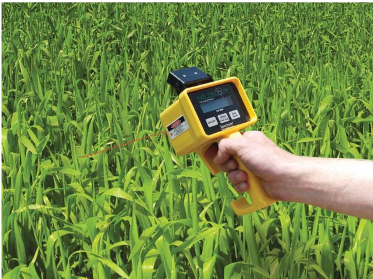
The NASA-derived, point-and-shoot FieldScout meter can take chlorophyll measurements from individual leaves or across a canopy, providing valuable information for nutrient management of crops and turf grass.
