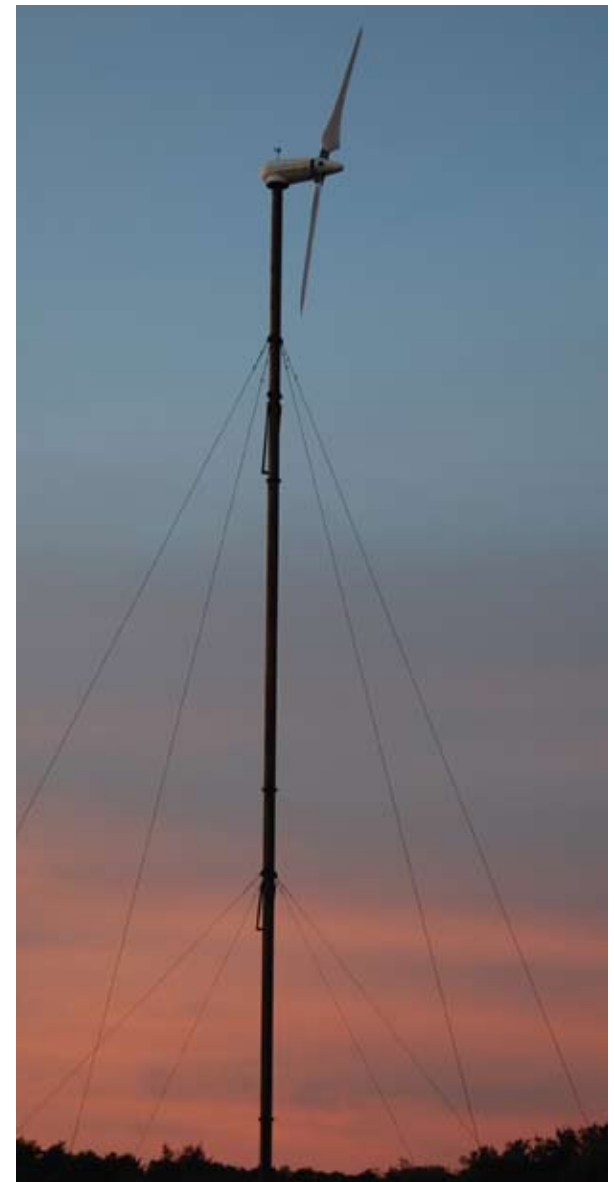
Aerostar’s wind turbines are stall regulated, a feature enabled by the Viterna model.
