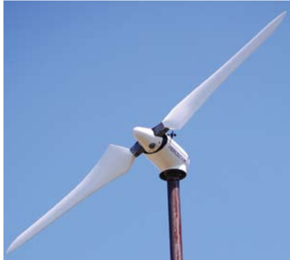
The teetering, two-bladed rotor of Aerostar's wind turbines is similar to that of NASA's early designs.
