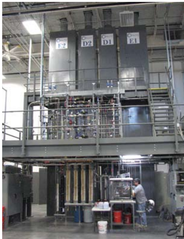
By increasing the size of its fluidized bed reactors, seen here, SouthWest NanoTechnologies Inc. (SWeNT) increased its carbon nanotube production capacity while at the same time lowering cost.
