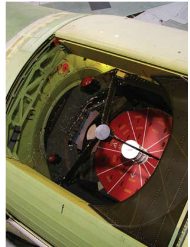
The infrared (IR) telescope of the Stratospheric Observatory for Infrared Astronomy (SOFIA) peers through the opening in the fuselage of its Boeing 747 mothership.
