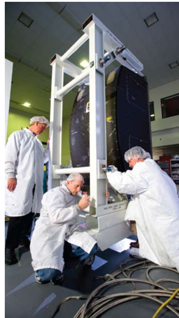
NASA engineers prepare one of the two ISS Water Recovery System racks for transport. The system will help the station accommodate six crewmembers.
