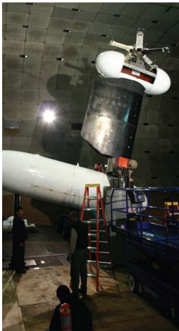
Engineers prepare the SMART rotor hub for wind tunnel testing. The rotor's piezoelectric enhancements help control noise and vibration.
