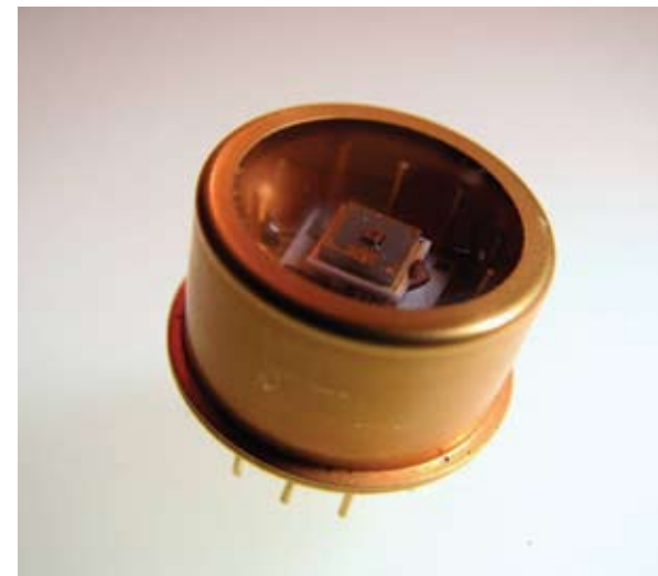
Amplification Technologies's NIRDAPD photomultiplier can sense infrared light down to individual photons, without the cooling required by other infrared sensors.
