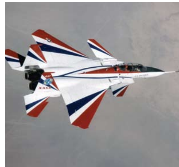
Originally an F-15 fighter, NASA's NF-15B Intelligent Flight Control System aircraft has validated adaptive control concepts that may improve commercial aviation safety.
