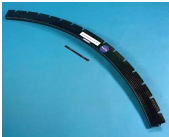
PETI-330 was used in resin transfer molding to fabricate this F-frame. Composite manufacturing is simpler and faster with PETI-330, because it needs only a one-step curing process.
