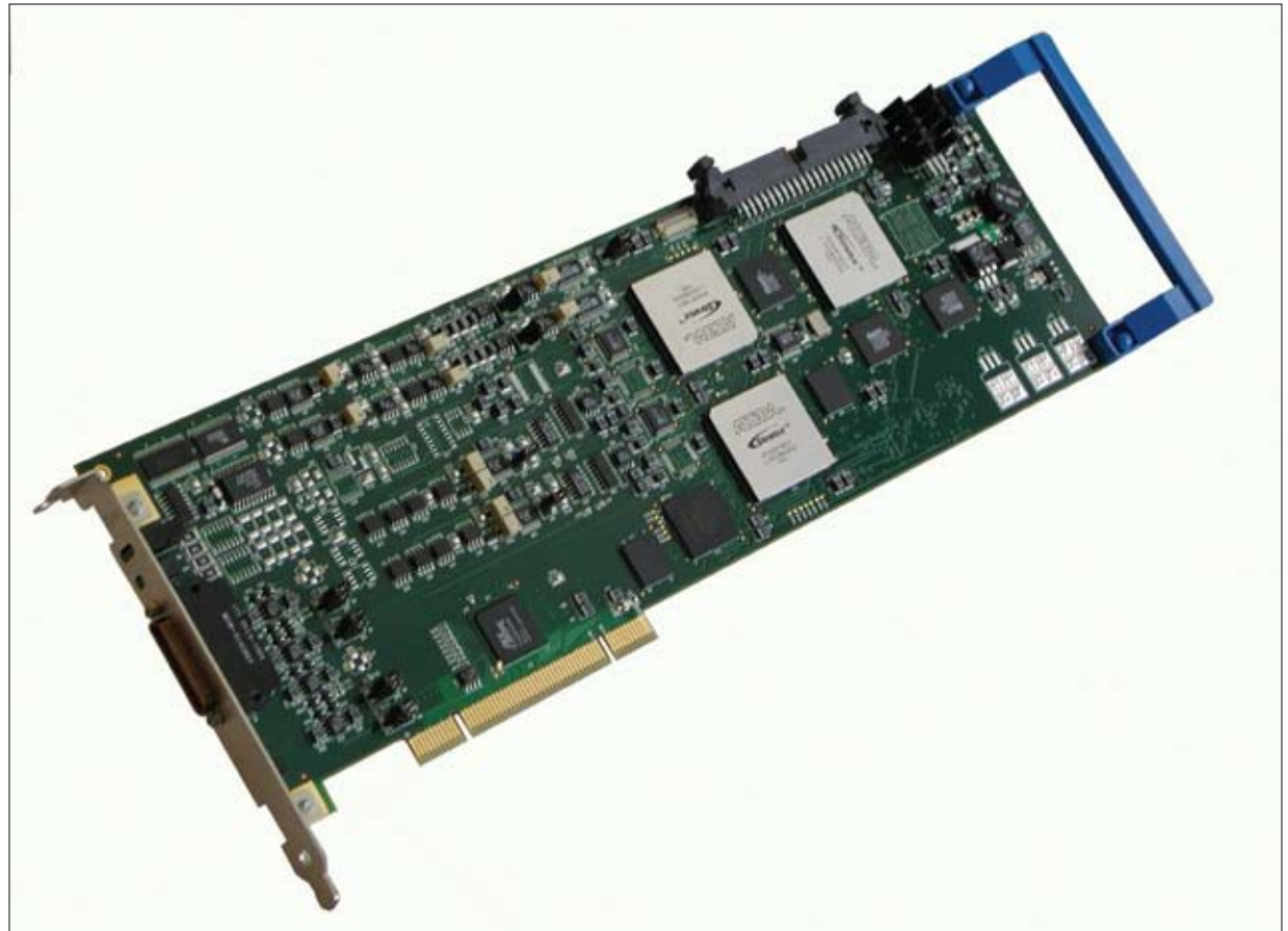
The TarsusPCM board—enhanced through Ulyssix's partnership with NASA—translates raw telemetry data into understandable measurements for engineer analysis, playing an essential role in satellite launch and ground support, as well as the testing of remote-controlled drones and jet engines.
