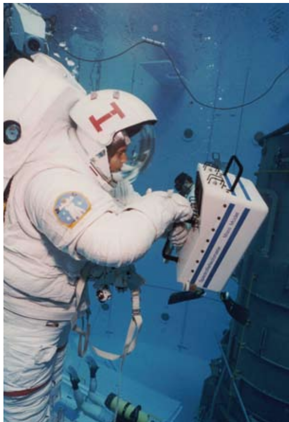
During training exercises, an astronaut uses a mockup of a space-portable spectral reflectometer, an instrument for measuring the thermal properties of surfaces in space.
