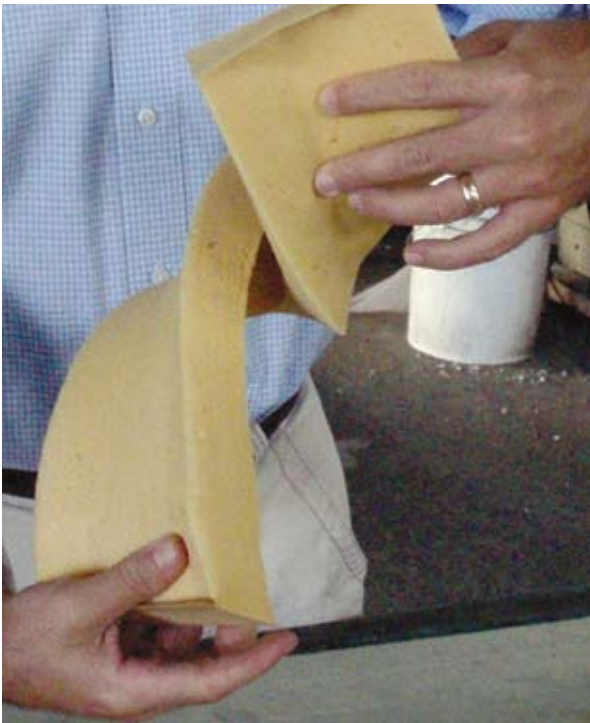
The commercial Polyshield foam is flexible, flame-retardant, and provides excellent thermal and acoustical insulating properties.
