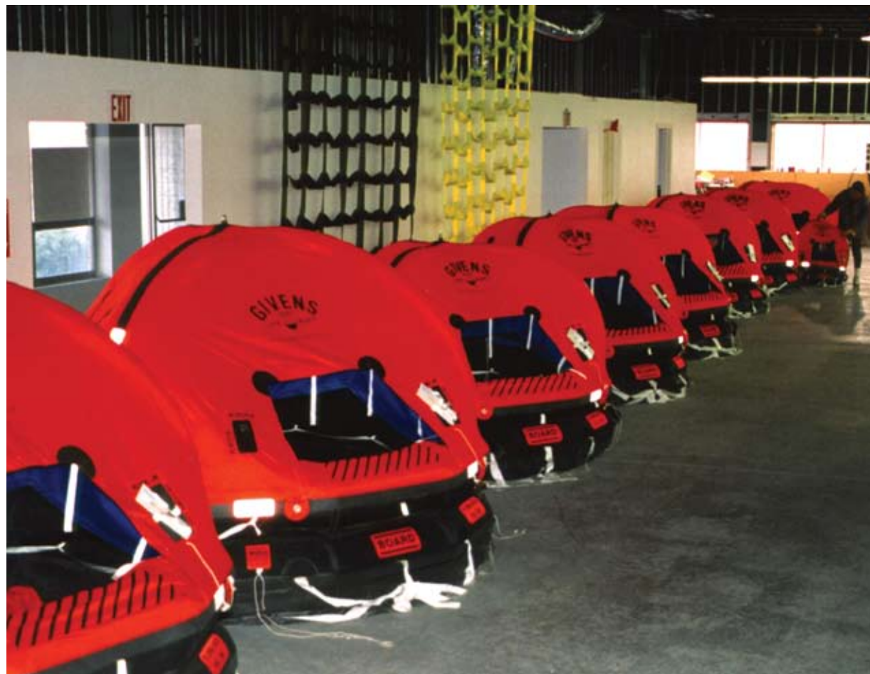
Available in a variety of sizes, the Givens Buoy Life Raft can be used on small sailboats or large fishing vessels and fully self-inflates in under 12 seconds.
