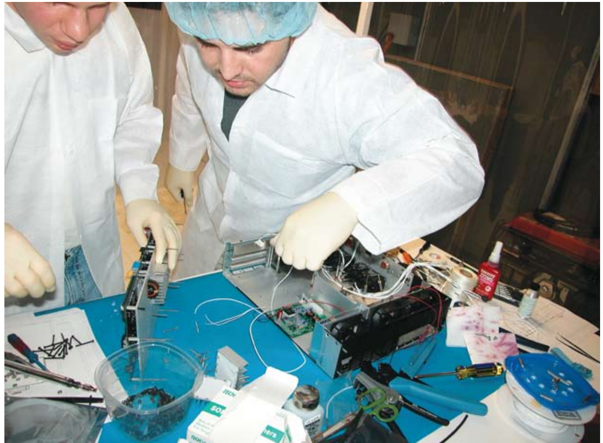
Engineering students assemble the AgCam power data controller in a clean room facility at the University of North Dakota.
