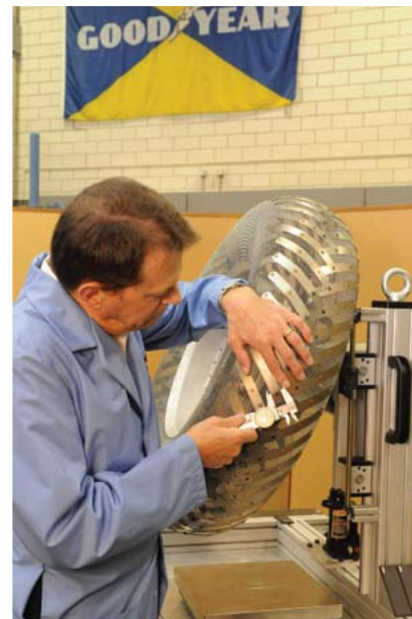
Goodyear Tire and Rubber Company is working with Glenn Research Center through a Seed Fund to create non-pneumatic tire technologies for use on the Moon.
