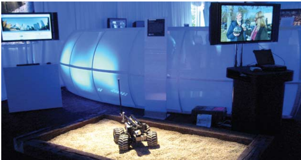
The Multi-function Agile Remote Control Robot (MARCBot) pictured here on display at WIRED NextFest, an annual showcase of innovative technologies transforming the world, is a tele-operated reconnaissance robot developed to identify explosives from a safe distance.
