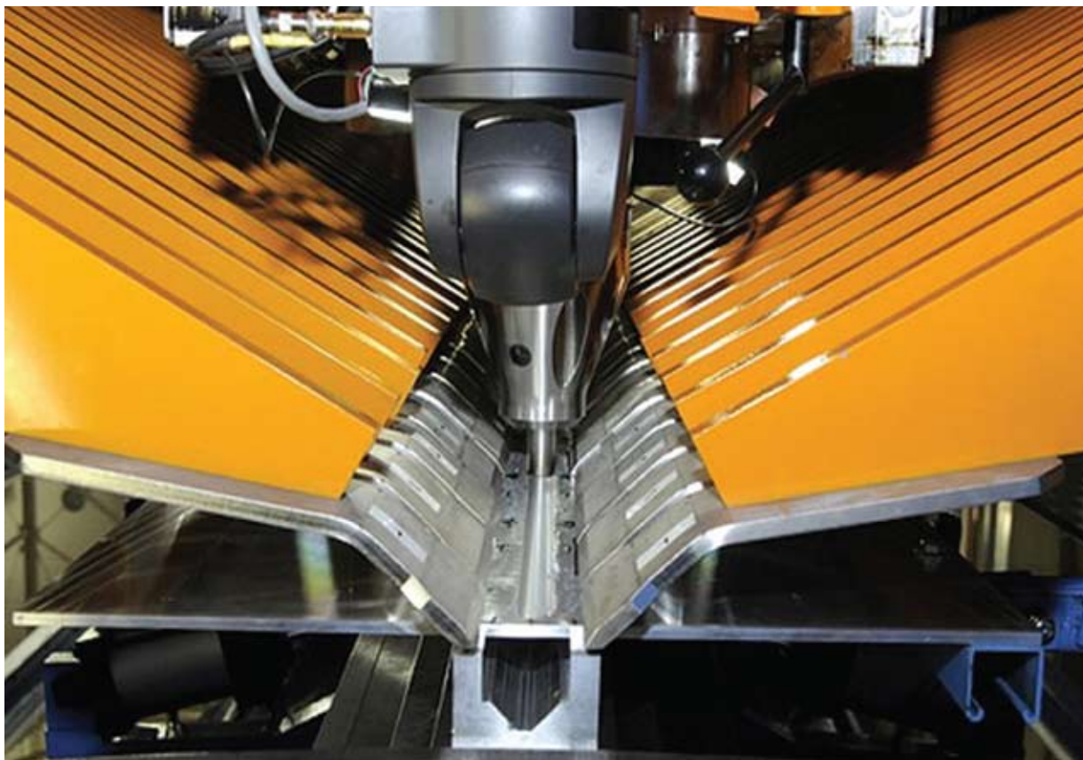
To fabricate the Ares I rocket for the Constellation Program, NASA employs friction stir welding (FSW) techniques. FSW has been enhanced by the invention of an auto-retractable pin tool by Marshall Space Flight Center engineers.
