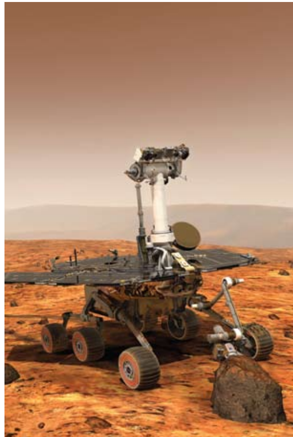
Concern over static electricity damaging components on Mars rovers Spirit and Opportunity led scientists to add grounding wires to the base of the rovers' antennas.
