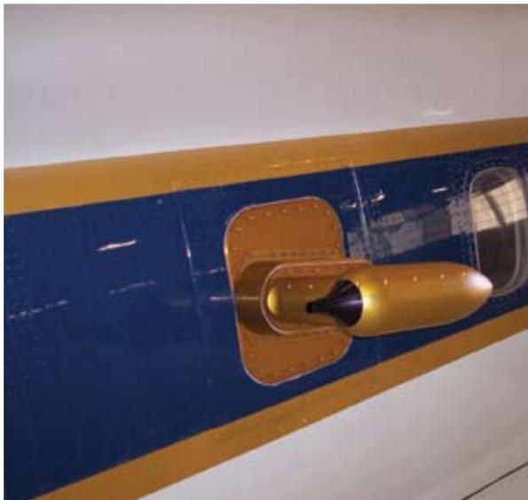
Stratton Park Engineering Company Inc. (SPEC) installed its Cloud Particle Imager (CPI) on NASA's High Altitude Research Program aircraft. Research facilities around the world have since used the commercially available CPI to further atmospheric study.
