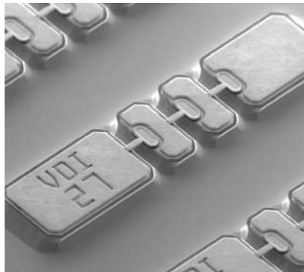
Virginia Diodes Inc. (VDI) has found commercial success with its high-frequency integrated diodes, which are key components in VDI's vector network analyzer (VNA) extenders.
