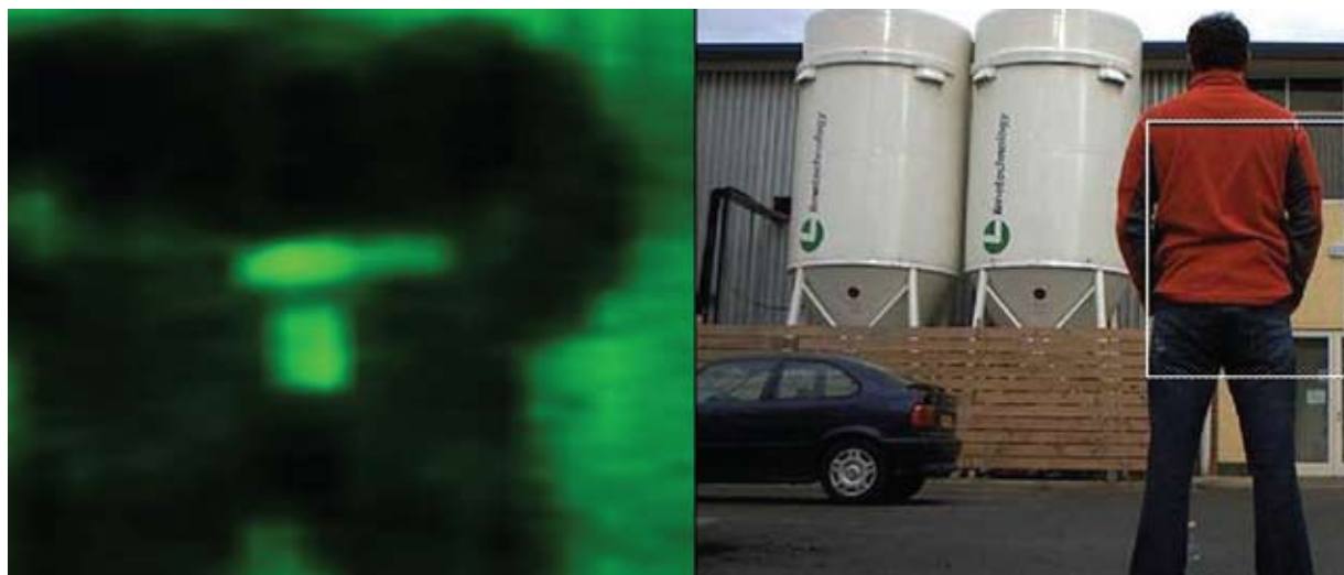
New security imaging products use the VDI diodes to detect passive terahertz waves, which can reveal images hidden behind common materials. The image on the left, returned from the security system, shows a gun hidden under the man's jacket.
