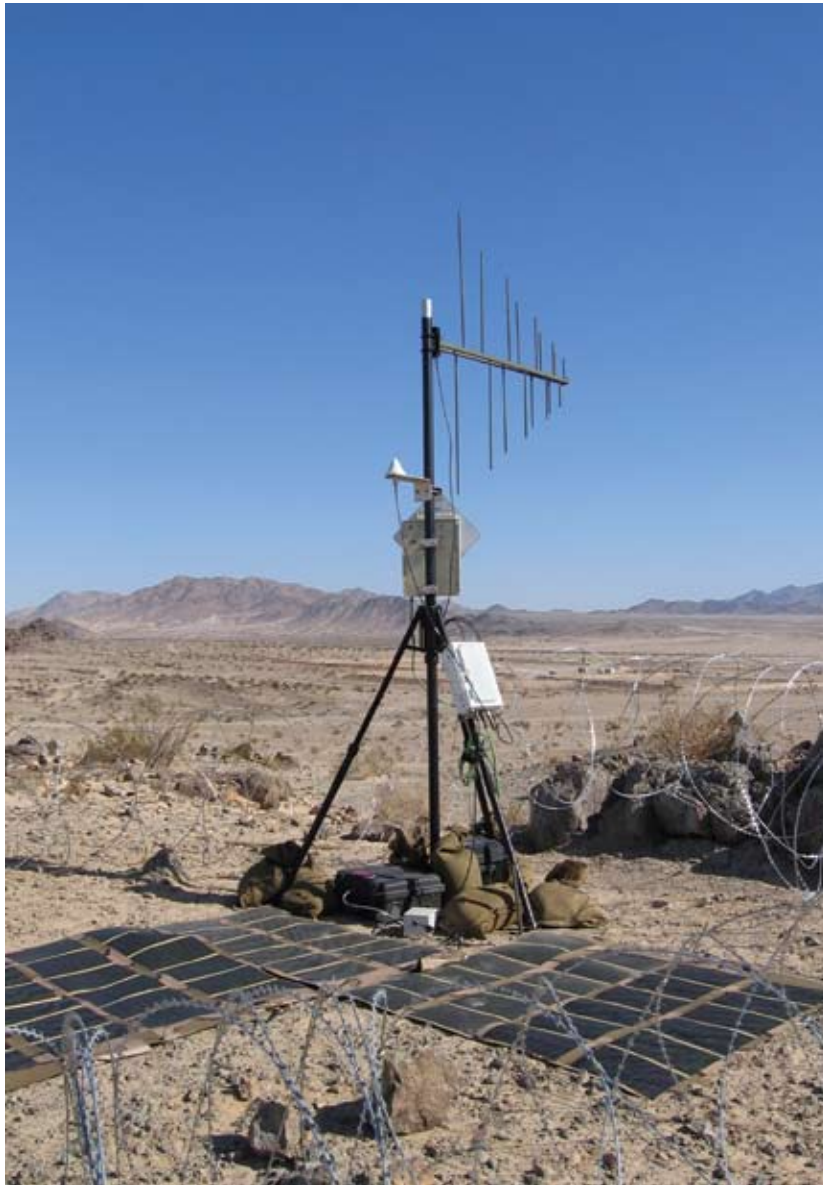
Soneticom's Lynx Location System is an electromagnetic interference geolocation system that relies on NASA-derived receiver components.
