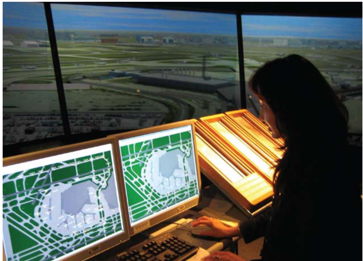
The Aviation Systems Division at Ames Research Center has contributed to surface automation research by helping to develop surface traffic management systems, which are decision-support tools designed to aid surface traffic planning.
