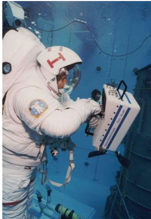
During training exercises, an astronaut uses a mockup of a space-portable spectral reflectometer, an instrument for measuring the thermal properties of surfaces in space.
