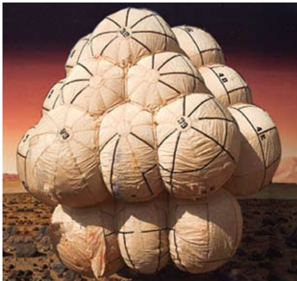
The Mars Pathfinder's airbags incorporated multiple layers (up to four, depending on the location of the airbag) of lightweight fabric. When Pathfinder landed on Mars, the vehicle and its delicate payload were protected by 24 inflated spheres woven by Warwick Mills Inc.
