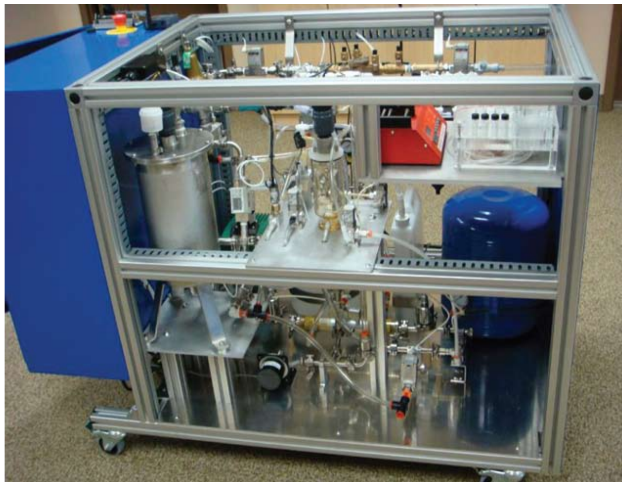
Early Warning’s analyzer feeds a concentrated water sample to its biosensor, providing rapid pathogen detection.
