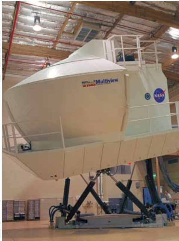
Astronauts and pilots receive line oriented flight training (LOFT) in simulators, such as the one shown here. LOFT prepares crews for both routine and hazardous situations through highly realistic simulations.
