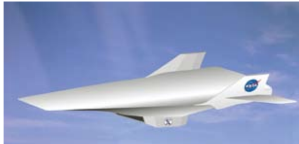
Artist's concept of the air-breathing X-43A Hypersonic Experimental Vehicle, or "Hyper-X." NASA is using software by companies such as TechnoSoft Inc. to design these supersonic combustion ram-air compression jets (scramjets).
