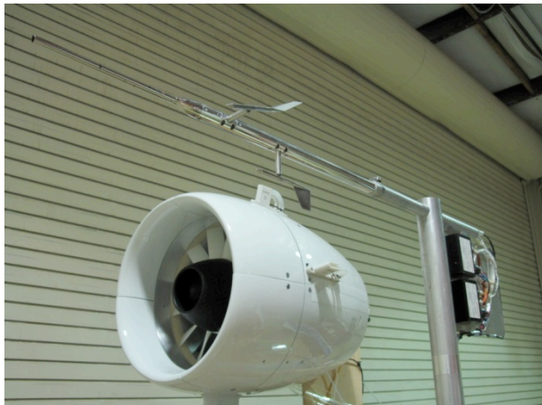
Airdata probe (pitot, static, alpha, beta)
