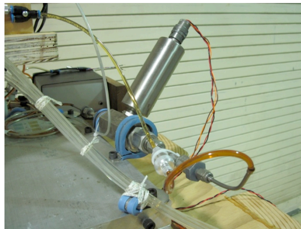
Volumetric fuel flowmeter
