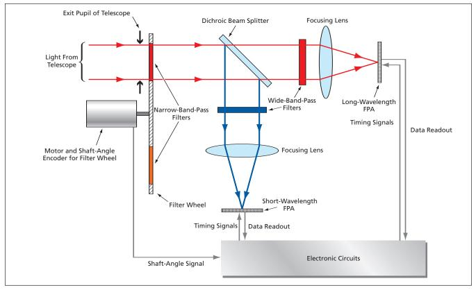
Figure 1. The **Dichroic Beam Splitter** and associated optics and electronics make it possible to utilize light from the telescope, even when the light beam straddles two adjacent narrow-band-pass filters. Light passed by one of these filters goes to one FPA; light passed by the other filter goes to the other FPA.
