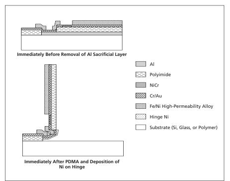
Figure 2. The Cantilever Remains Horizontal during most of the fabrication process. It is released by etching away the aluminum sacrificial layer, then raised to its perpendicular orientation by PDMA.
