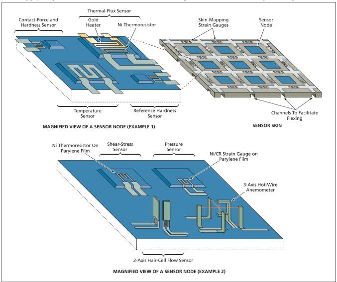
A Sensor Skin contains an array of sensor nodes, each node containing multiple sensors that measure different quantities. The sensor nodes shown here are examples only: the variety of potential sensor-node designs is practically unlimited.
