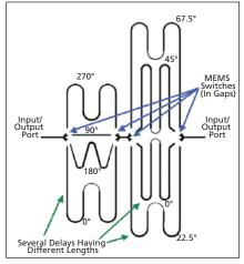
Figure 2. **MEMS Switches** are used to connect the input/output ports to one of the two delay lines to obtain one or the other of two different amounts of phase shift.
