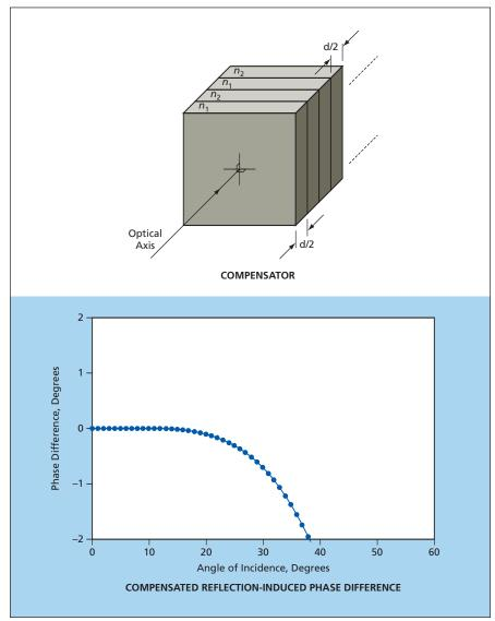
Figure 2. A **Coating Comprising Alternating Thin Dielectric Layers** having different indices of refraction would exhibit form birefringence that could be exploited to compensate for anisotropy like that of Figure 1.
