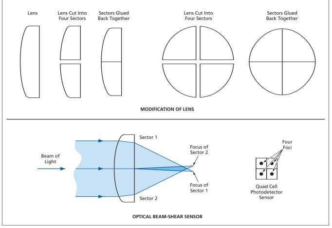
An Optical Beam-Shear Sensor can be made from a lens and a quad-cell photodetector.
