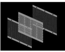
Metal Skeletal Layers Are Patterned to obtain desired properties — in this case, to make them easily stretchable in the vertical direction but not in the horizontal direction. To complete the fabrication of a composite skin according to the invention, these metal skeletal layers would be embedded in an elastomeric sheet.
