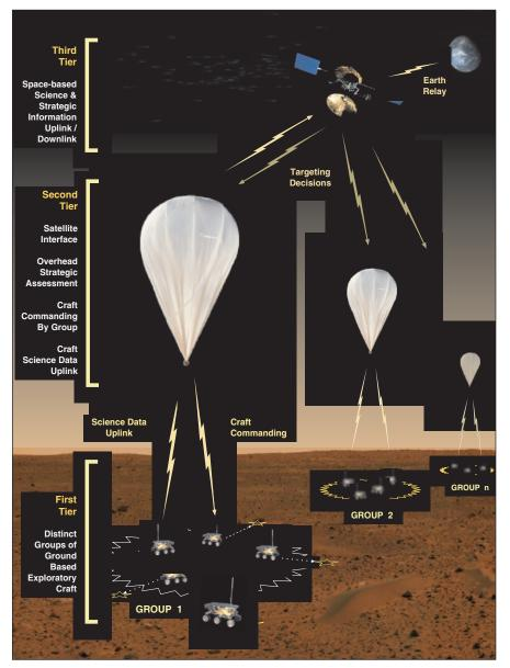
A Balloon-Borne Unit would supervise the maneuvers of multiple rovers from an overhead perspective.
