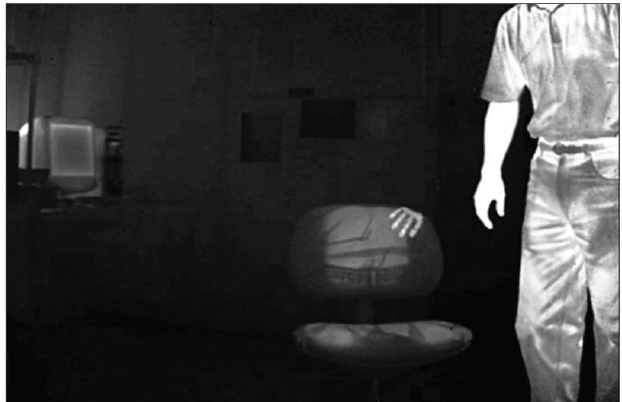
**This Image Was Generated From One Frame** of video readout, at frame rate of 30 Hz, from the camera described in the text.
