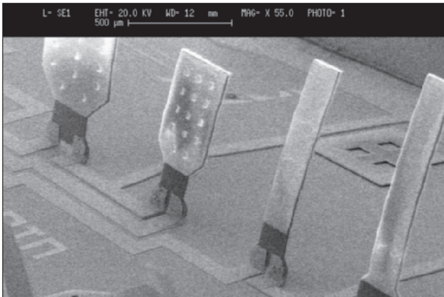
Figure 1. Artificial-Hair-Cell Flow Sensors shown in this scanning electron micrograph have several different widths as well as different heights ranging from 0.6 to 1.5 mm.
