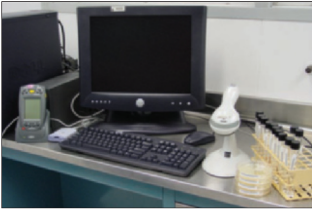
The Bar-Code System Hardware includes a personal computer, a desktop bar-code scanner (on the right by tubes and plates), and a PDA with a built-in bar-code scanner (left of the keyboard).
